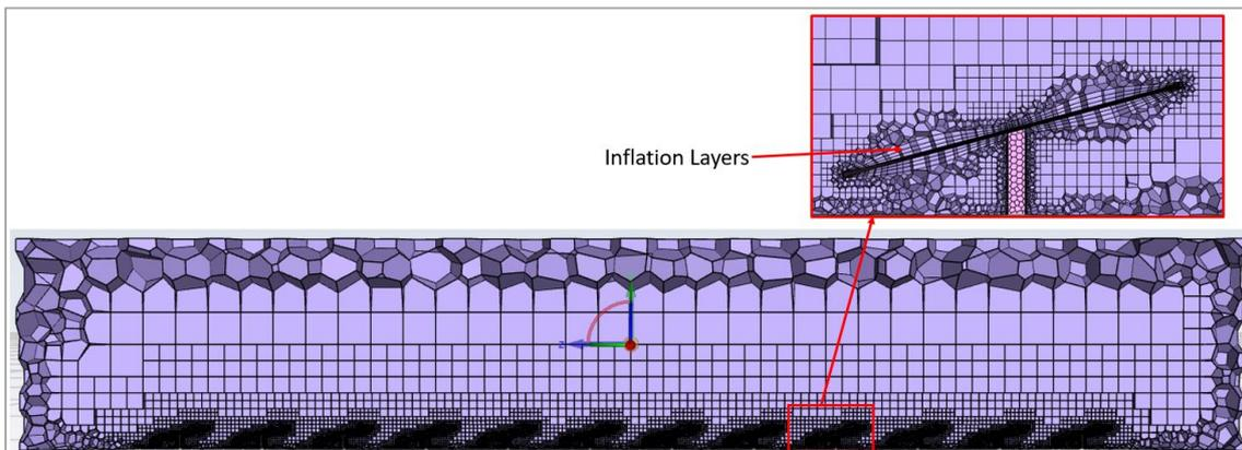
**Figure 5-5: Meshed Model Cross-section**
