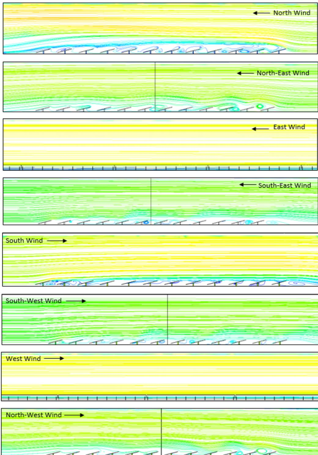
**Figure 7-1: Velocity streamlines from eight wind directions**
